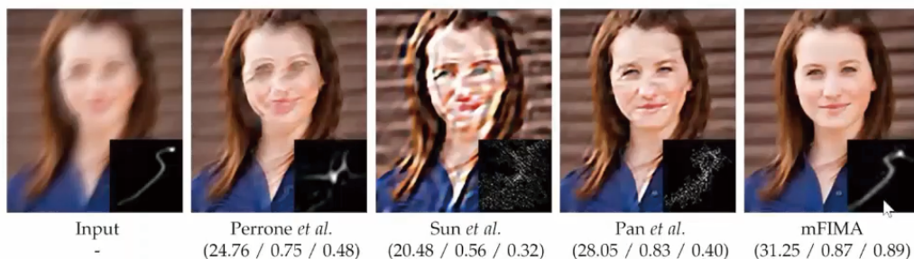
Fig. 9. The blind image deconvolution results of mFIMA with comparisons to state-of-the-art approaches on blurry facial image with 3% Gaussian noise. The quantitative scores (i.e., PSNR / SSIM / KS) are reported below each image.
